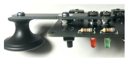
☐ Insert the last ¾" screw into the hole nearest the center of the PCB arm, and lightly secure with a nut.
